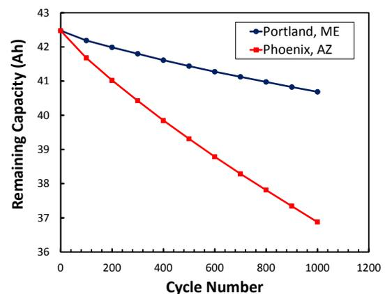
Figure 2: Capacity fade as a function of cycle number for hot (Phoenix, AZ) and cold (Portland, ME) environment with US06 drive cycle.
