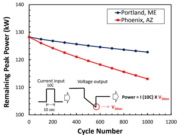
**Figure 3: Power fade as a function of cycle number for hot (Phoenix, AZ) and cold (Portland, ME) environment. Power is characterized at 40% SOC for a 10 sec 10C-rate pulse at 25°C.**
