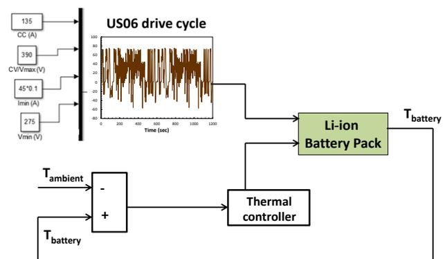
Figure 1: System block diagram with US06 drive cycle and control logic on battery pack temperature.
