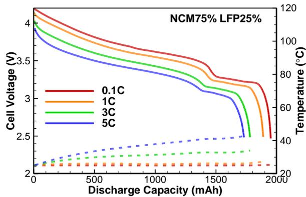
Figure 2 Discharge performance of Li-ion cell using blended NMC-LFP cathode
