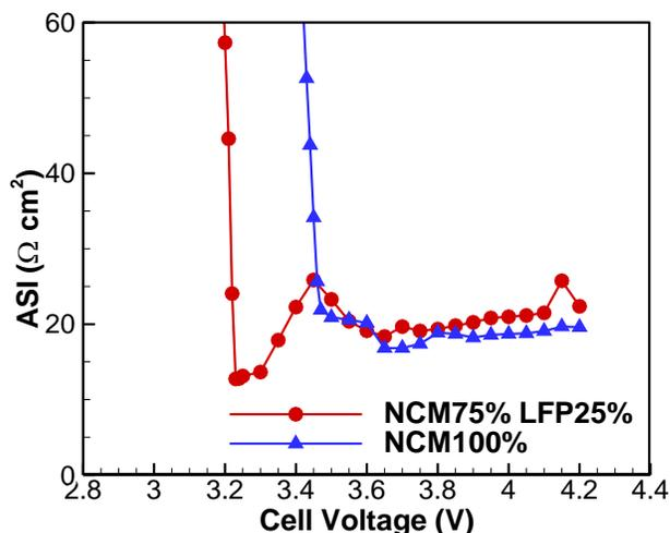
Figure 1: Simulated electrochemical impedance for NMC-LFP blended cathode (red line) and NMC cathode (blue line)
